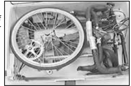
Fig. 27 Front wheel placement.
