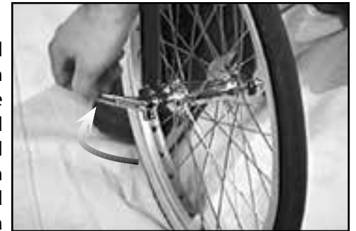
Fig. 2 Setting quick release tightness.
