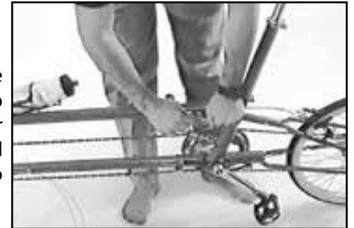
Fig. 6 Detach rear brake housing.
