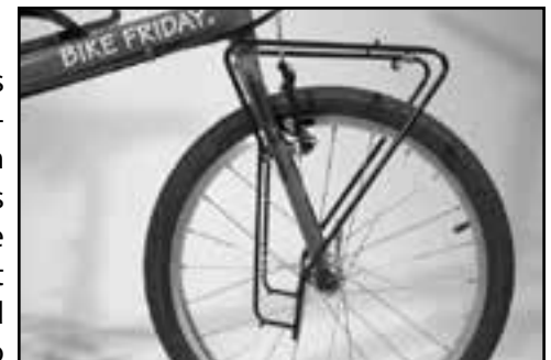
Fig. 6 Completed front rack.
