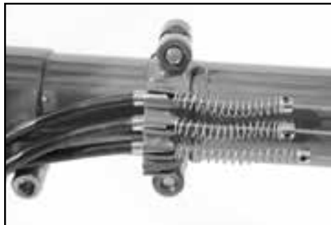
Fig. 11 Cable guide ring and springs.
