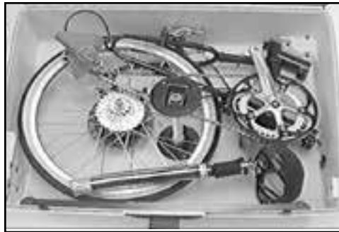
Fig. 36 Crush protector placement.
