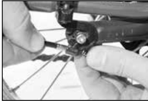
Fig. 20 Drum brake cable housing stop.
