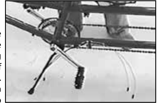
Fig. 4 Lower cables on bottom tube.
