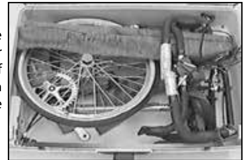
Fig. 28 Bottom & top tube placement.
