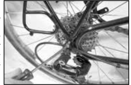
Fig. 4 Mount rack legs to drop outs.
