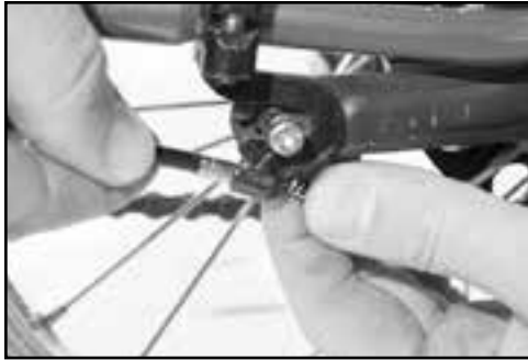
Fig. 15 Drum brake cable housing stop.
