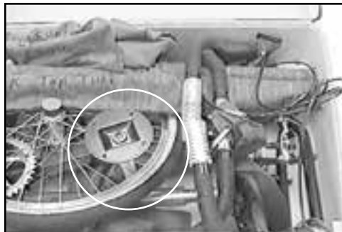
Fig. 31 Crush protector placement.
