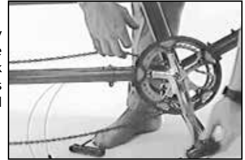
Fig. 11 Derail timing chain.
