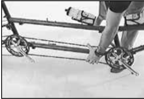
Fig. 21 Squeeze chain to add slack.
