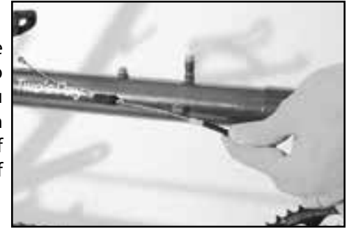
Fig. 2 Disconnect brake cable splitter.
