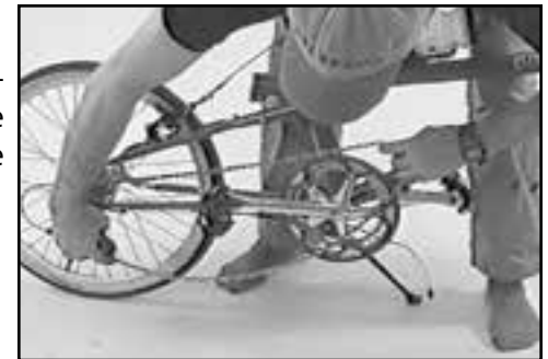
Fig. 18 Drive chain installation.
