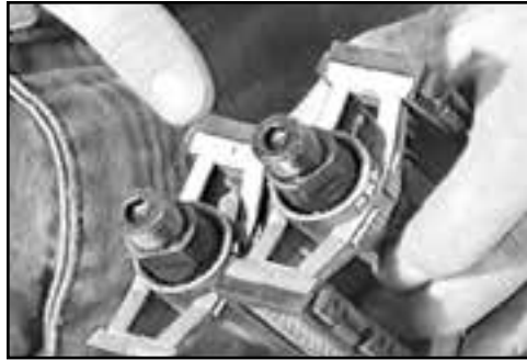
Fig. 40 Check pedals for threading.
