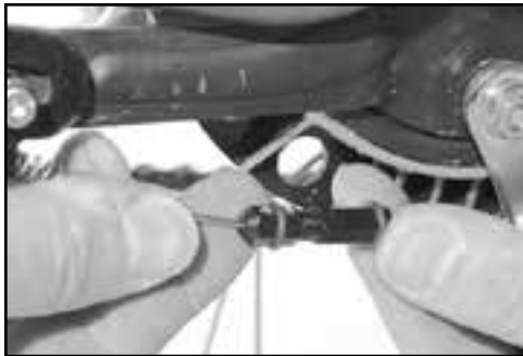
Fig. 16 Drum brake cable splitter.
