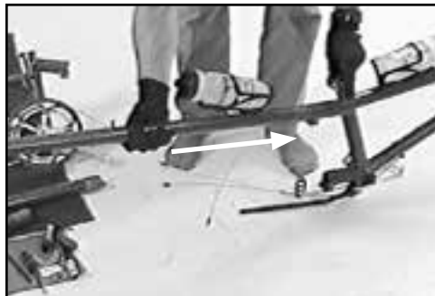
Fig. 5 Mid top tube inserted into socket.
