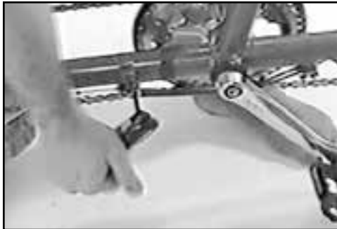
Fig. 9 Loosen all center clamp bolts.
