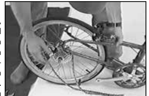
Fig. 18 Remove rear wheel.
