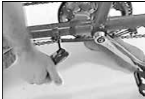
Fig. 9 Loosen all center clamp bolts.
