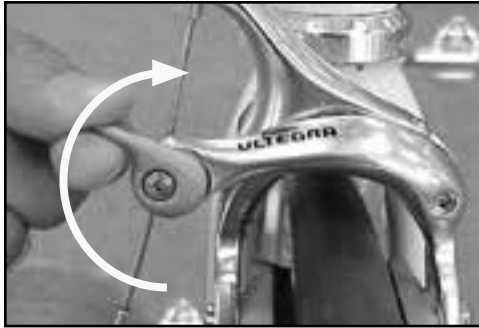
Fig. 34 Opening side-pull brake.
