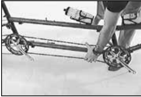
Fig. 21 Squeeze chain to add slack.
