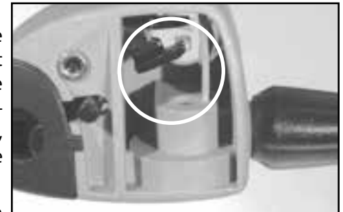
Fig. 6a Shifting fork up, button stuck.
