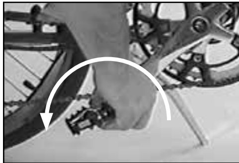
Fig. 2 Remove pedals (loosen in opposite direction for left pedal).
