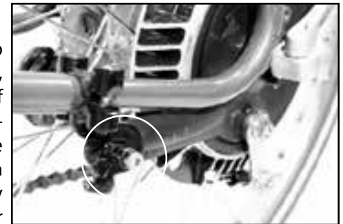
Fig. 14 Drum brake arm mounted.
