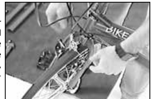
Fig. 6 Open both brakes.
