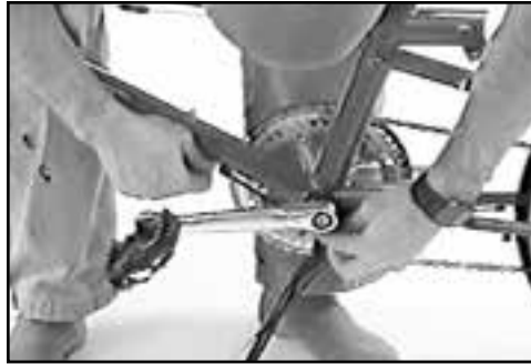
Fig. 19 Connect control cables.
