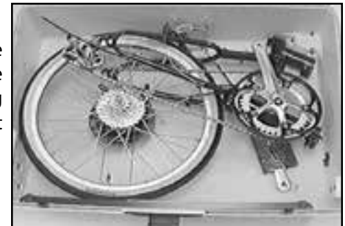
Fig. 34 Rear wheel placement.
