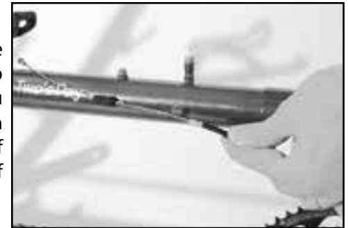
Fig. 2 Disconnect brake cable splitter.
