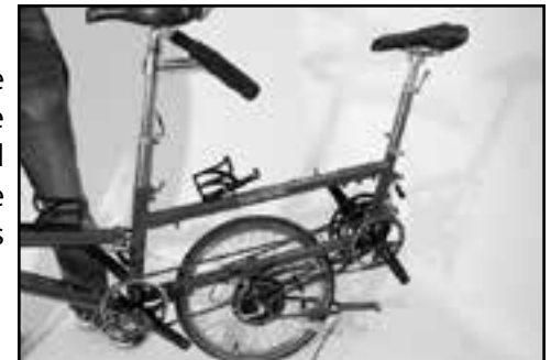
Fig. 3 Fold under rear end.
