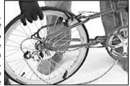
Fig. 12 Install rear wheel.
