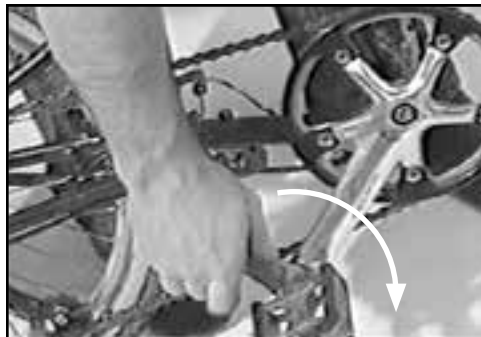
Fig. 41 Tighten pedals (tighten in opposite direction for left pedal).
