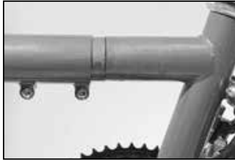
Fig. 9 Frame halves properly joined.
