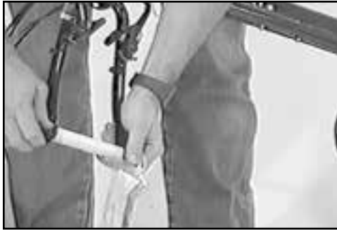
Fig. 33 Remove fork spreader.
