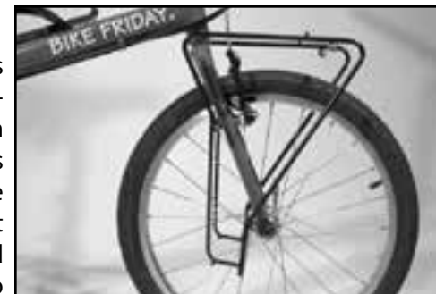
Fig. 6 Completed front rack.
