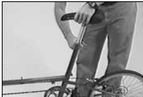
Fig. 3 Remove saddle and seat post.
