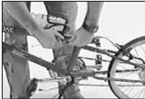
Fig. 20 Connect rear brake.
