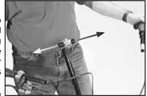
Fig. 10 Remove captain's handlebars.
