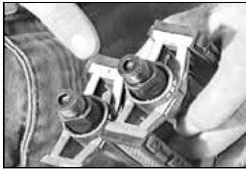
Fig. 40 Check pedals for threading.
