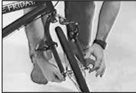
Fig. 7 Remove front wheel.
