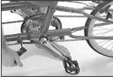
Fig. 14 Loosen frame clamps.
