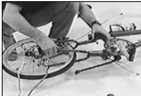
Fig. 15 Attach rear end to frame.
