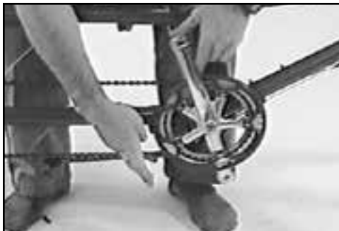
Fig. 15 Remove timing chain.
