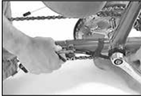
Fig. 7 Detach lower control cables.
