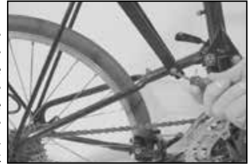
Fig. 5 Attach rack stays to wish bone.
