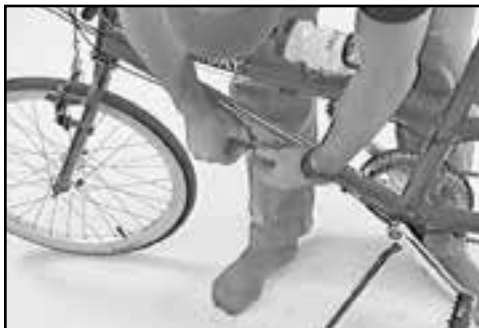
Fig. 2 Disconnect front cable splitters.
