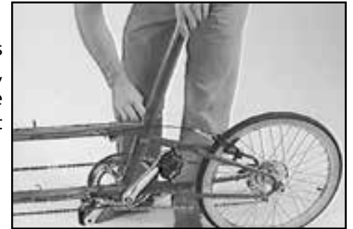
Fig. 5 Remove seat masts.
