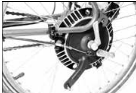
Fig. 21 Drum brake hub out of frame.
