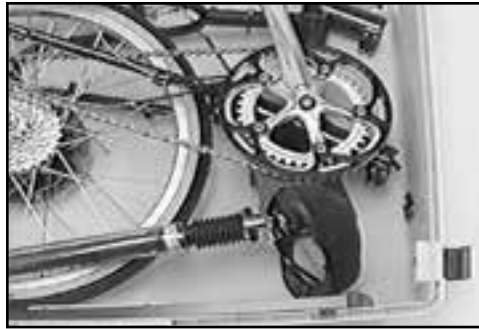
Fig. 35 Saddle & seat post placement.
